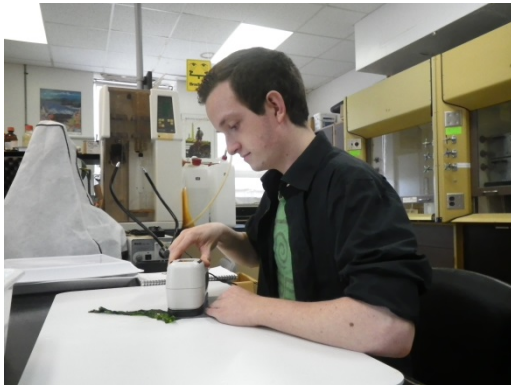
Kasper Brandt using a spectrophotometer to measure the colour of recently harvested Ulva lactuca (photo credit: Caroline Longtin).
